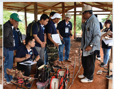
Figure 22: Practicing resistivity measurement in the salt factory ground, instructed by Mr Somkiat Kongsuwan
