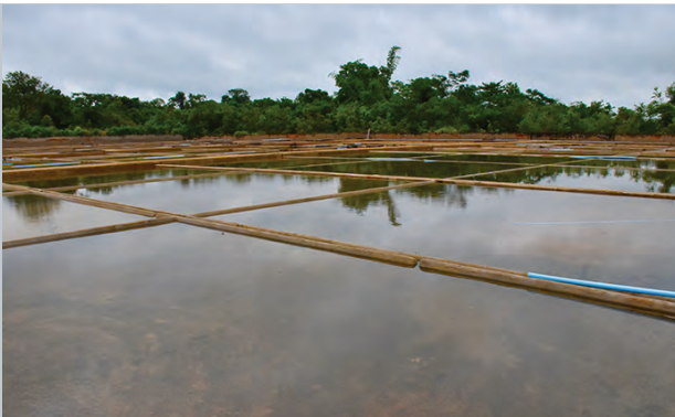
Figure 18: Sundry pond for salt precipitation.
